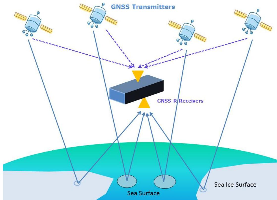
Figure 1. GNSS-R for sea ice detection
